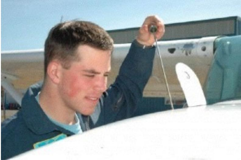
*There's a lot more to checking the dipstick than just noting the oil level. The appearance of the oil is at least as important as its quantity.*
