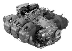
As the engine warms up moisture from engine and oil vaporizes and is vented overboard through the breather tube. The breather tube may freeze shut causing the engine's internal pressures to increase until
