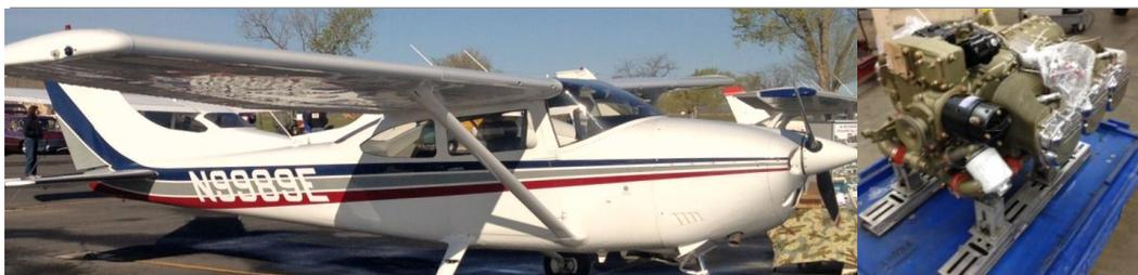
improvements. The basic O-470 engine consisted of two separate configurations identified by the shape and style of the cylinder head. Early models incorporated a parallel valve (also known as a straight valve) cylinder head, large, round intake port and small, two-bolt, exhaust port and stack assembly. The present day standard issue is the angle valve cylinder having a greater cylinder fin area and the induction and exhaust ports with a four bolt pattern.
