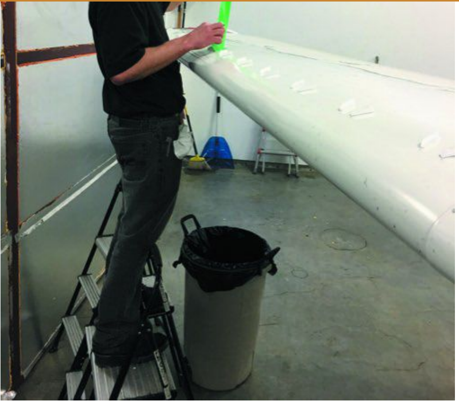
Removing the template after VG installation on a wing.
