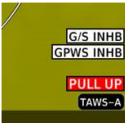
TAWS-A alert inhibit annunciations appear at the bottom right of the display.
